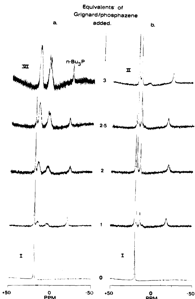
Figure 6. Changes in the ^{31}P NMR spectrum following the addition of increasing amounts of CH_3MgCl to a 1:8 ratio mixture of [n-Bu_3PCuI]_4 and (NPCl_2)_3 . (a) Spectra of the reaction mixture before the addition of 2-propanol. (b) Spectra after the addition of 2-propanol.
